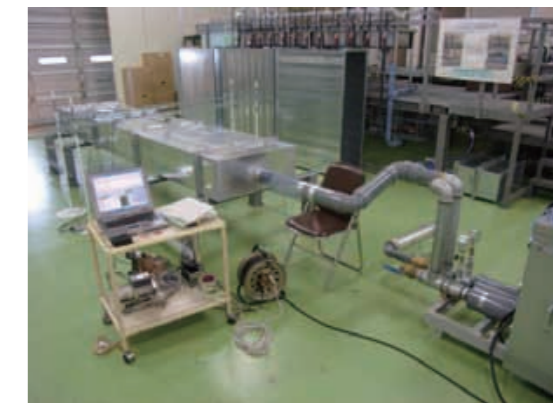
Performance evaluation testing of laminate ducts
