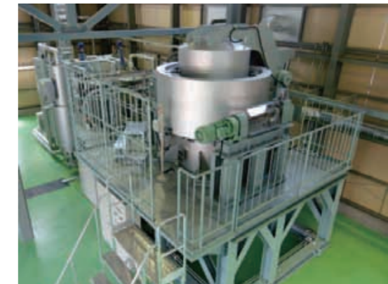
Japan's largest supercritical CO2 cleaning and recycling equipment
