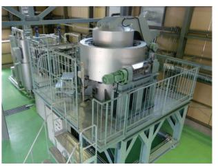
Japan's largest supercritical CO2 cleaning and recycling equipment
