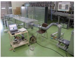
Performance evaluation testing of laminate ducts
