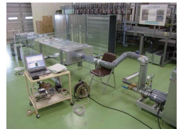
Performance evaluation testing of laminate ducts
