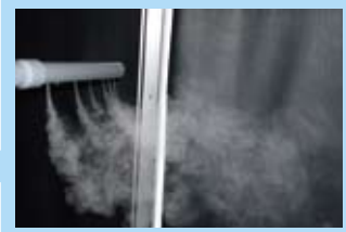
▼ One-way flow of air when door is opened
