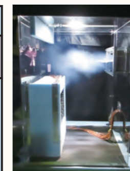
Mock-up of the air conditioning machine room allows for examination of airflow during ambient air cooling
