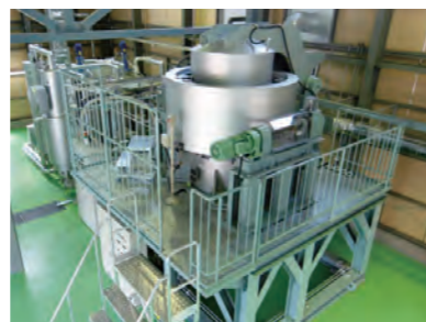
Japan's largest supercritical CO 2 cleaning and refurbishment equipment
