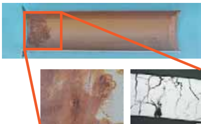
Example of corrosion analysis (Piping sampling inspection)
