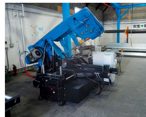
Fully automated bandsaw (pipe cutting machine)
