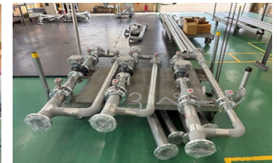
Processed air-conditioning piping systems
